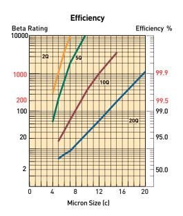
Notes: Multipass test run @ 80 gpm to 50 psid terminal - 5 mg/l BUGL.
